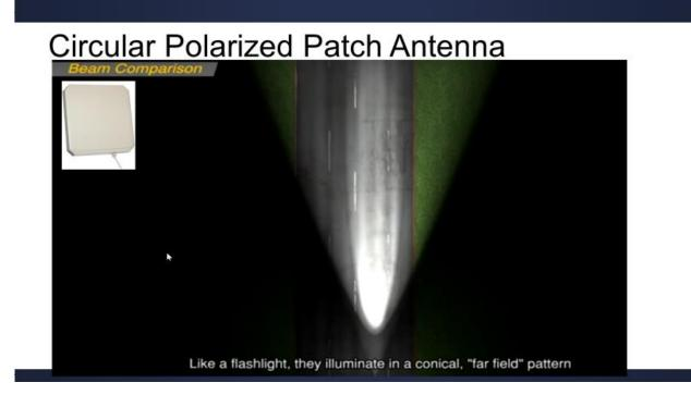
The circular patch antenna projects a far beam in a conical pattern which, when used in dock door portal applications, lends itself to cross-reads and stray reads - reading tags on assets other than those going through that particular doorway.
