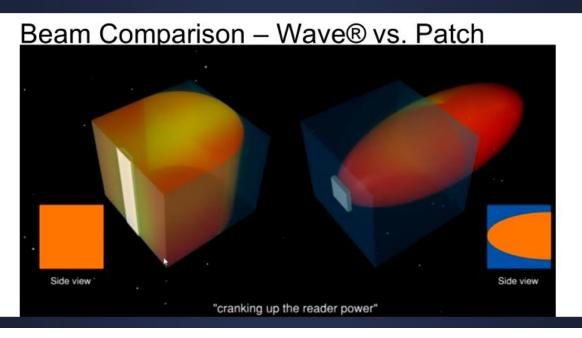
The Wave® Antennas are unique in covering all three tag orientations within a user defined zone up to a 10x10x10 foot zone. The Wave® antenna design creates a wide-angle lens effect which covers all three polarizations at once and are designed to work in high fading and multipath environments to provide superior UHF zone coverage.
