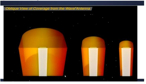
The SLS smartPORTAL™ enclosures include antenna back planes to direct signal into the designed read zone and eliminates adjacent dock-door reads while providing floor-to-top-of-door coverage at all RF-transmitted power levels.
