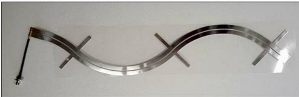
NeWave's Wave antenna—two of which are contained in each smartPORTAL—is designed to generate a uniform RF field.
